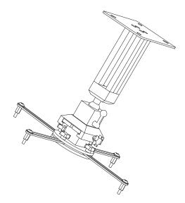
WARNING: This arm mount is intended to support projectors with a maximum weight of 26 lbs. If your projector does not have mounting nuts embedded in the bottom, it cannot be attached to this arm mount. THIS ARM MOUNT IS INTENDED AS A CEILING MOUNT ONLY.A QUALIFIED PROFESSIONAL SHOULD BE USED TO PROPERLY INSTALL THIS UNIT TO THE CEILING. RECORDEX DOES NOT RECOMMEND THE USE OF POWER TOOLS AND WILL NOT BE LIABLE FOR THE IMPROPER USE OR INSTALLATION OF ITS PRODUCTS.
