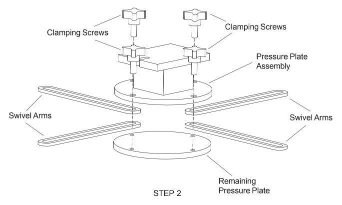
Align pressure plate assembly, swivel arms and remaining pressure plate as shown. Loosely tighten together using the clamping screws. The number of arms you attach (either 3 or 4) will be determined by the number of mounting nuts embedded in the bottom of your projector. Lay your projector on its top (protected by a soft cloth or other suitable protection) to expose the bottom and the embedded mounting nuts.
